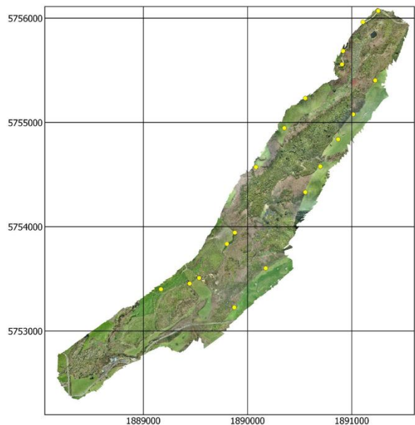
Figure 3: Waikite calibrated thermal infrared orthophoto (top) and RGB orthophoto (bottom). Yellow dots show location of ground control points. Map Datum NZGD2000.
