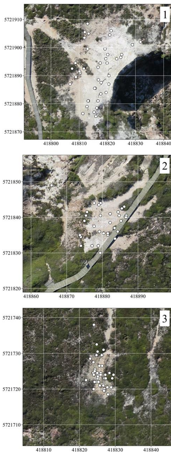
Figure 4: At Karapiti, soil CO 2 flux and shallow temperature measurement locations (white points \pm 5 m) are overlaid on high-resolution drone aerial orthophoto (4cm GSD). Note areas correspond to those in Figure 5.
