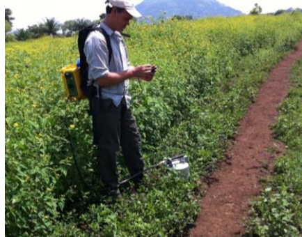
Figure 4: Soil CO 2 flux measurement at San Jacinto, July 2011. CO 2 flux analyser is worn as a backpack, and accumulation chamber placed over soil (Harvey et al, 2011).
