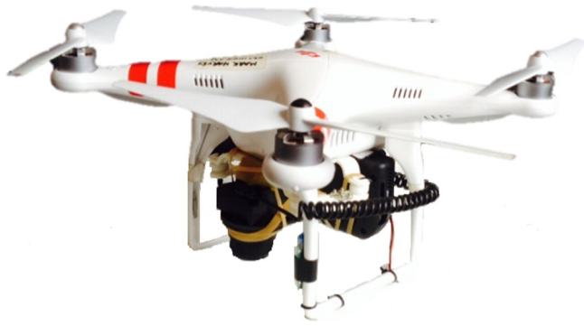
Fig. 1. DJI Phantom 2 Vision Plus quadcopter modified with ICI thermal camera and UAV module.
