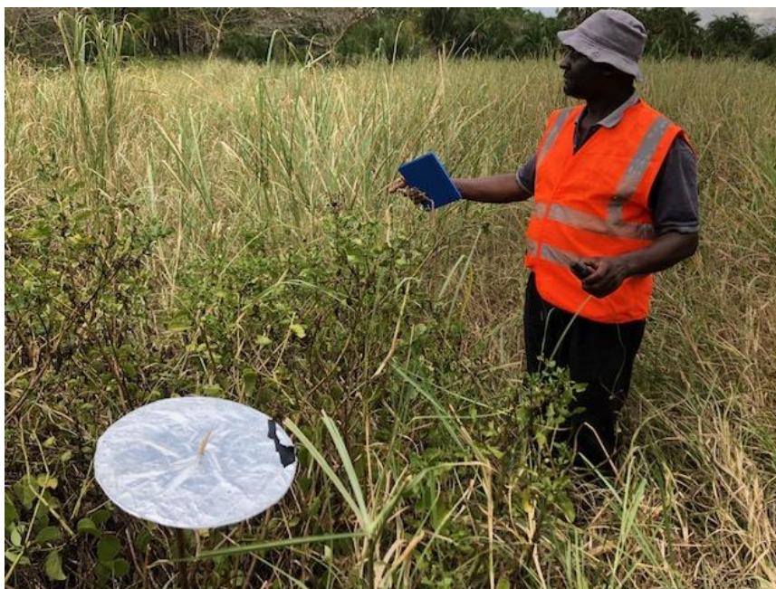
Figure 5: GCP made from a 12” vinyl record covered with aluminium foil.
