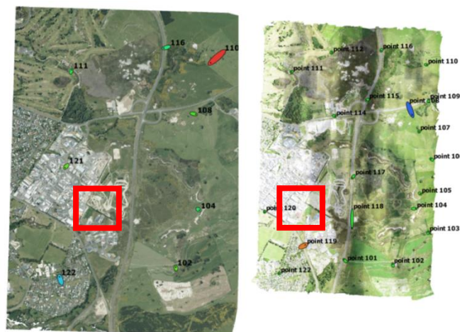
Figure 2: Dense point clouds from crewed aircraft survey 2017 (left), and from the 2018 UAS survey (right). Red square shows approximate location of Crown Rd subsidence bowl.
