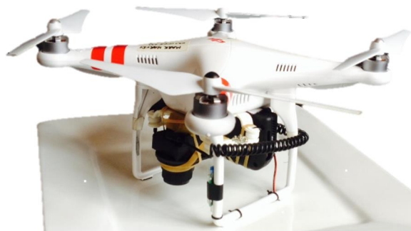
Figure 1: DJI Phantom quadcopter modified with ICI thermal camera
