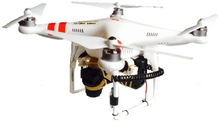
Figure 1 DJI Phantom 2 Vision Plus quadcopter modified with ICI thermal camera and UAV module
